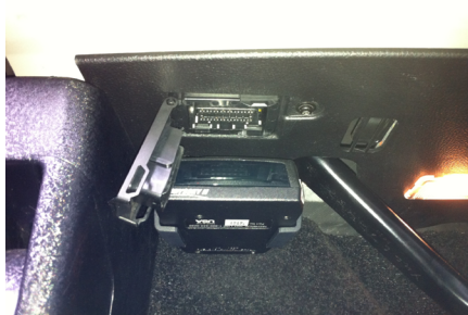
Figure 19. OBDII Connector, L319, L320, L322 2007 onwards, L359, L538, L405, L494
