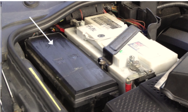
Figure 105. Battery fuse holder location
