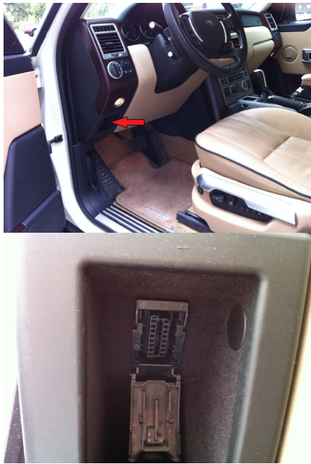
Figure 20. OBDII Connector L322 2002-2006
