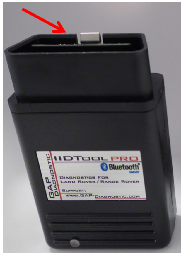
Figure 2. OBDII connector allowing connection of the IIDTool to a vehicle
